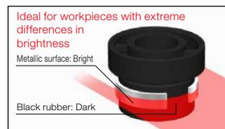
HDR mode creates a composite image from two images taken with different shutter times. This function is useful for workpieces with areas of high contrast such as reflective metal surfaces.
