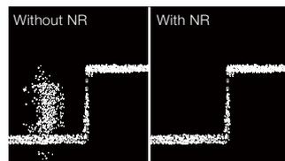
NR mode creates a composite image by amplifying an image of the bright areas and combining it with an image of the dark areas. This feature reduces noise such as ambient light.
